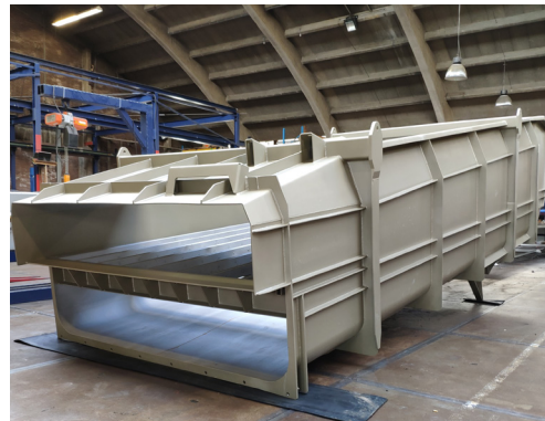
Rubber Lining Project : T-REX60 thickness 20 mm, ± 30 square metres
